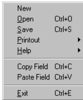
The first section of this menu offers choices to clear the screen and restart the program, open and save calculations, print the results, and access the help screen. The *Change Units* option converts between English and Metric units. In the second section, *Copy* and *Paste*, are used to transfer data to or from other fields and the Conversion Calculator. *Exit* shuts down the heat exchanger sizing module.
